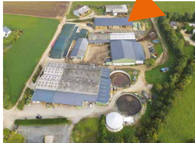
In addition to photovoltaic panels, the GAEC des Papineaux, which hosted our Wide Angle days in 2022, has also installed a methanisation micro-plant that produces biogas from the farm's waste.
